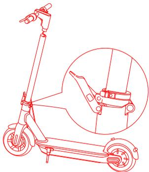
2. Slide the handle onto the stem. Be aware of the correct orientation.
