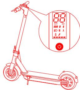
1. Power on the KickScooter and check the battery level. Charge the KickScooter if the battery level is low.
