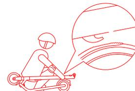
Then fold the handlebar down until it locks into the rear fender.
