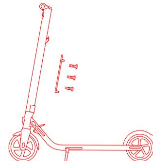
3. Install the external battery on the rail and fix it with the M4 (20mm) screws (2 pcs) and M3 screw (1 pcs), provided with this product. After they are properly installed, block the screw holes with the rubber stopper.
