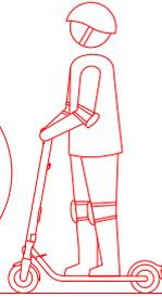
3. Put your other foot on the footrest to keep both feet stable. Press the throttle on right hand to speed up when you are balanced.
