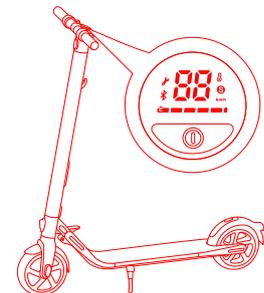
1. Power on the scooter and check the indicator lamp power level. Charge the scooter if the battery level is low.
