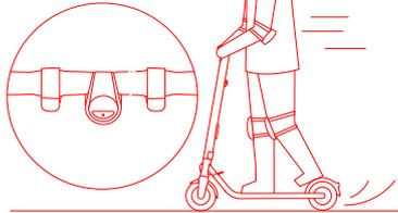
4. Slow down by releasing the throttle. Squeeze the electronic brake and stamp the fender with foot at the same time for a sudden brake.
