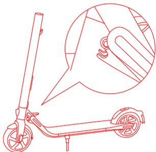
3. Install six screws (two on each side) with the included hex wrench.
